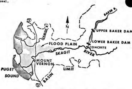
The recommended plan calls for an additional 58,000 scre-feet of storage space to be provided by 15 November. The pool would be kept below elevation 707.8 from 15 November, except during an actual flood event, until 1 March. Use could be made of the reservoir's full capacity for hydroelectric power generation by 1 April. See page 15 for the existing and proposed flood control rule curves, including actual drawdowns for 1970-1973.
