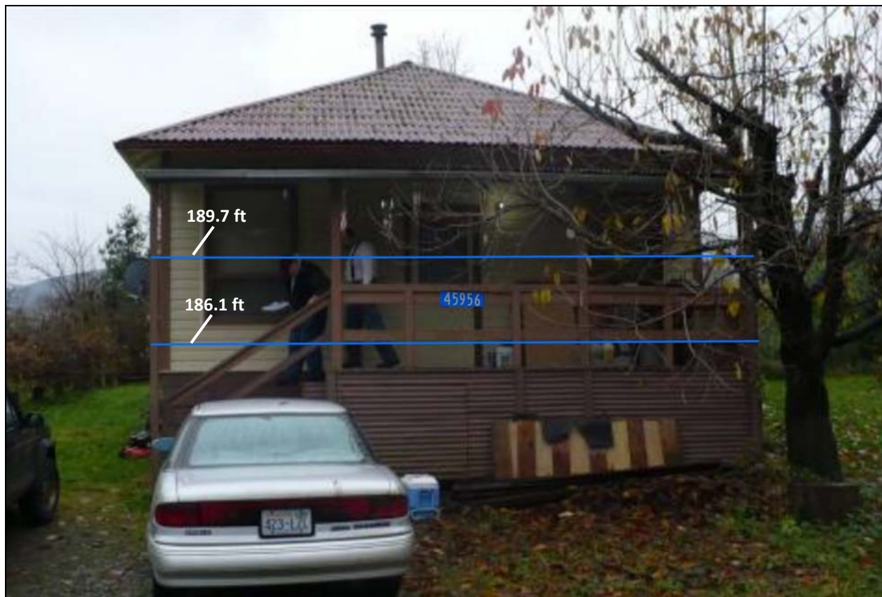
Figure 17. 45956 Albert Street, showing December 1921 water level as inferred from Concrete Herald report (186.1 ft), and estimated water level corresponding to a discharge of 228,000 cfs (189.7 ft)
